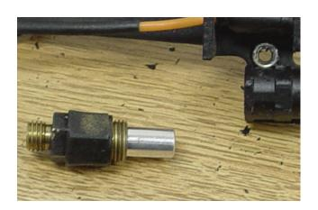
Remove the burner orifice unit as shown left, clean out the inside, and use a small piece of wire to ream out the gas jets in the burner orifices. Use a stiff wire brush to clean off the Thermocouple tip and the pilot burner.
