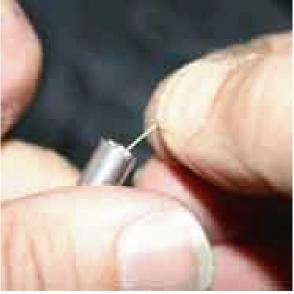
3 | Use a small wire or a straight pin to clean out the tiny gas jets inside the burner orifice. Blow the soot out of the inside of the burner orifice. Reassemble the unit using pipe thread to avoid gas leaks.
