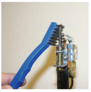
1 Shut off flame and let fixture cool until it is cool to the touch. Run a Dental Floss tooth pick or something small thru the slot in the tip, to clean the carbon buildup. Then use a steel brush to brush away debris or soot that may have gathered in area.
