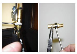
2 Remove the burner body from the bracket.
